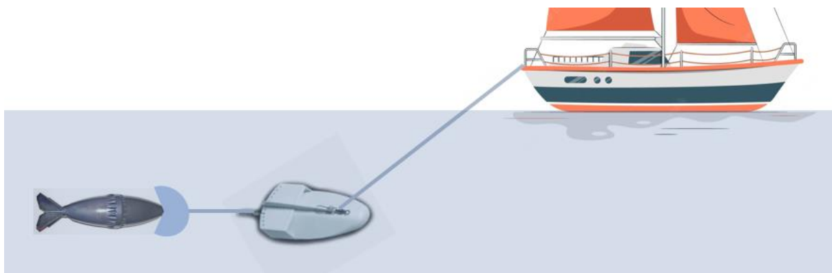
Fig. 6: The Whale-PAL is towed behind the boat on a 10m long stainless-steel line using a paravane at a water depth of 2-3m. In this way it blocks orca access to the rudder
